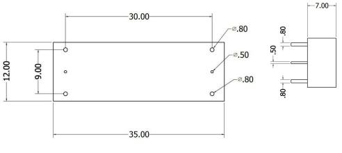
Unit in mm 1mm = 0.0394 inches Tolerance: +/- 0.2 mm
