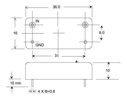
Unit in mm 1mm = 0.0394 inches Tolerance : +/- 0.2 mm
