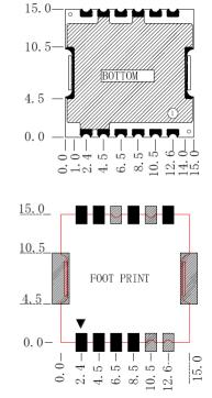
PLL1515BQ-FS-2296MHz-2490MHz-A 2296-2490MHz SMD Phase Locked Loop (PLL) Synthesizer
