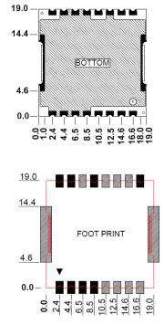
PLL1919BQ-FS-2050MHz-2080MHz-A 2050-2080MHz SMD Phase Locked Loop (PLL) Synthesizer
