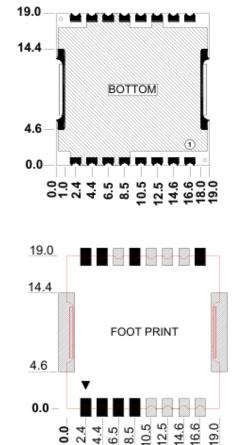
PLL1919BQ-SS-2110MHz-2140MHz-A 2110-2140MHz SMD Phase Locked Loop (PLL) Synthesizer
