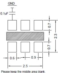
To ensure optimal oscillator performance, place a by-pass capacitor of 0.1µF as close to the part as possible between Vcc and GND pads
