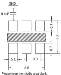
To ensure optimal oscillator performance, place a by-pass capacitor of 0.1µF as close to the part as possible between Vcc and GND pads
