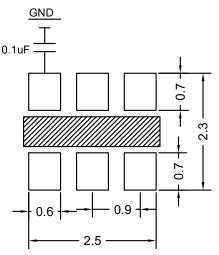
Please keep the middle area blank. Do not layout any lines in this space. To ensure optimal oscillator performance, place a by-pass capacitor of  $0.1\mu F$  as close to the part as possible between Vcc and GND pads
