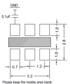
Do not layout any lines in this space. To ensure optimal oscillator performance, place a by-pass capacitor of  $0.1\mu F$  as close to the part as possible between Vcc and GND pads
