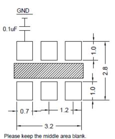
Do not layout any lines in this space. To ensure optimal oscillator performance, place a by-pass capacitor of 0.1µF as close to the part as possible between Vcc and GND pads
