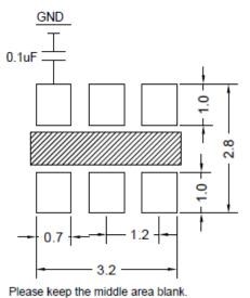
Do not layout any lines in this space. To ensure optimal oscillator performance, place a by-pass capacitor of  $0.1\mu F$  as close to the part as possible between Vcc and GND pads
