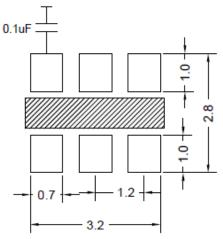
Please keep the middle area blank. Do not layout any lines in this space. To ensure optimal oscillator performance, place a by-pass capacitor of  $0.1\mu F$  as close to the part as possible between Vcc and GND pads
